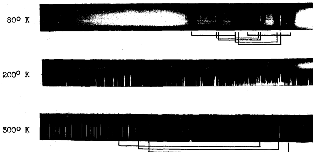
Fig. 7. Temperature effect in the 6300 Å multiplet of neodymium bromate. Contact prints from twenty-one foot grating plates. Lines fade out as the population of upper states decreases with lowered temperatures.
